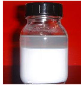
Fig. 2: Syneresis in an emulsion coating
