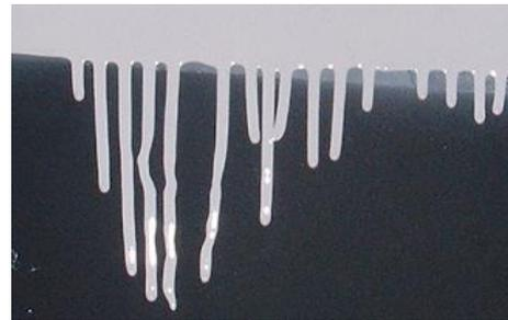
Fig. 3b: Waterborne emulsion coating with 'runners'
