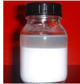
Fig. 2: Syneresis in an emulsion coating
