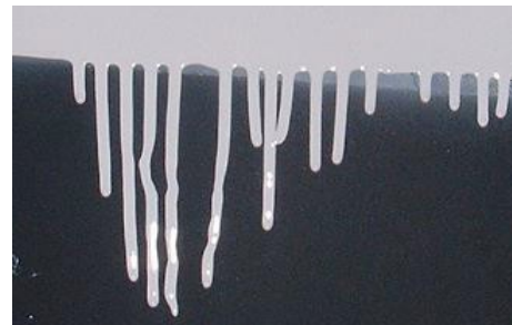
Fig. 3b: Waterborne emulsion coating with 'runners'
