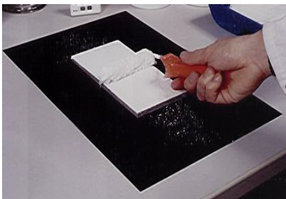
Fig. 4a: Roller-coated coating without adequate high shear thickener
