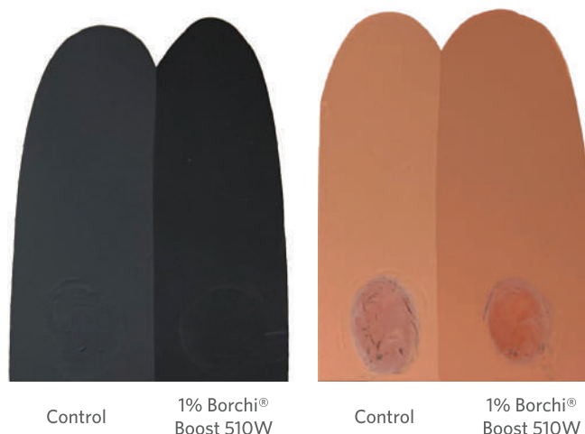
Figure 2: Borchi® Boost 510W enhances colour strength in decorative vinyl acetate ethylene emulsions tinted with universal waterborne colourants
